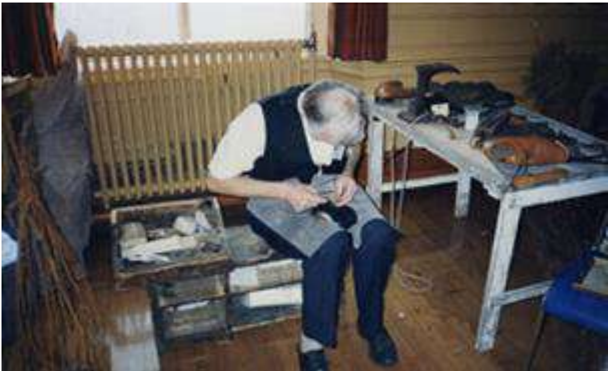
Ernie Reid sewing on leather soles by hand in the traditional manner using John Buchan's tools, and sitting on John Buchan's original shoemaker's stool.
